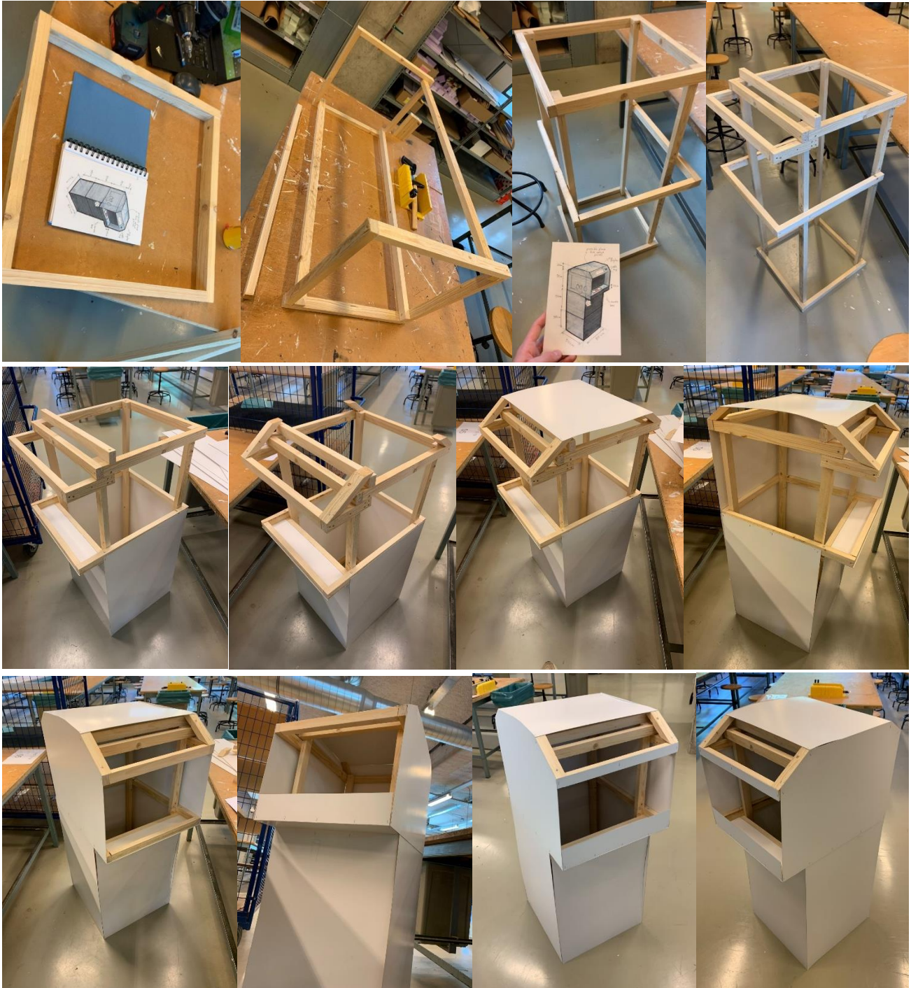
Figure 10, The preliminary design steps of the physical trash can.
